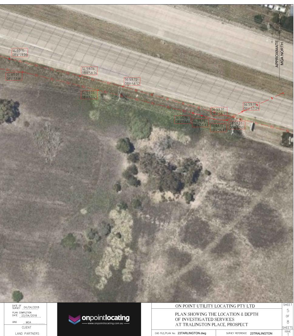
ELECTRONIC SUB SURFACE UTILITY ENGINEERING (SUE) DETECTION TECHNIQUES SUCH AS EM & GPR ARE INFLUENCED BY SSU TYPE & GROUND CONDITIONS. BEST PRACTICE DETECTION RATES ARE 80–90% AND DEPTH ACCURACY RANGES BETWEEN +/- 250MM FOR 90% OF READINGS WITH SIGNIFICANT OUTLIERS FOR THE REMAINDER.
