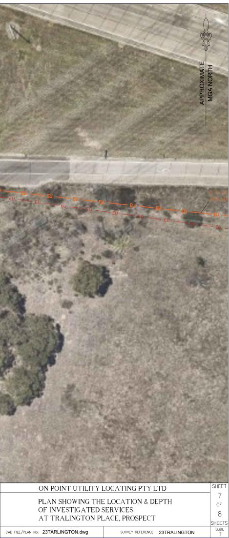
ELECTRONIC SUB SURFACE UTILITY ENGINEERING (SUE) DETECTION TECHNIQUES SUCH AS EM & GPR ARE INFLUENCED BY SSU TYPE & GROUND CONDITIONS. BEST PRACTICE DETECTION RATES ARE 80-90% AND DEPTH ACCURACY RANGES BETWEEN +/- 250MM FOR 90% OF READINGS WITH SIGNIFICANT OUTLIERS FOR THE REMAINDER.
